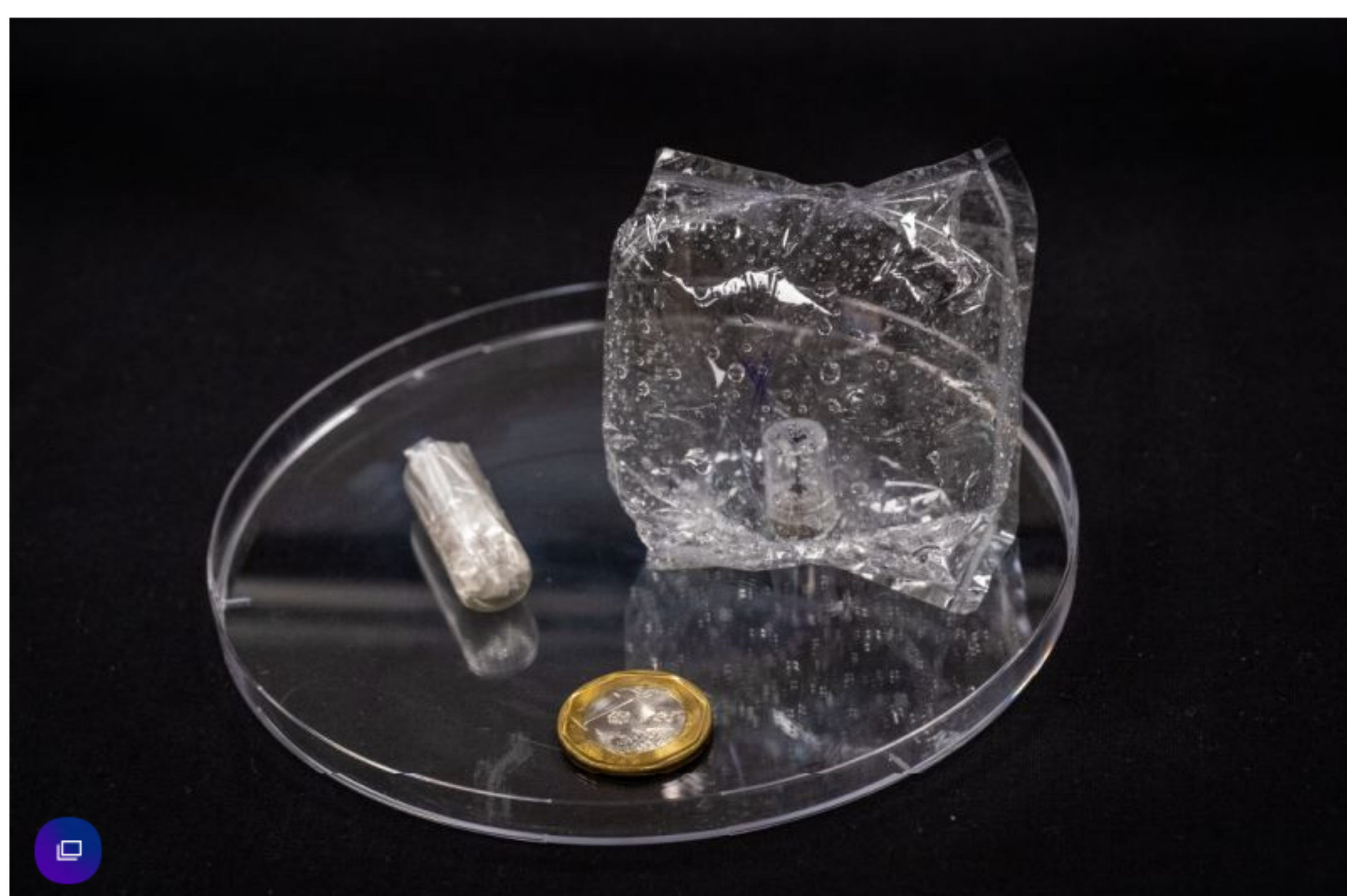
The EndoPil capsule is designed to be ingested orally with water and can be self-inflated with a handheld magnet to induce a "sense of fullness". (PHOTO: NTU)
