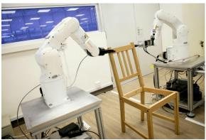
NTU SINGAPORE/AFP / Handout The device, consisting of two mechanical arms with grippers, starts the process by taking photos of the parts spread on the floor with a 3D camera, which is supposed to mimic the cluttered environment after flat-pack furniture is unboxed
