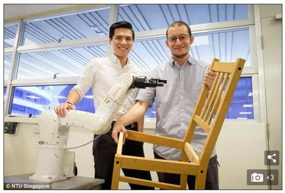
A pair of robot arms, able to bend in six different directions, used motion sensors and grippers to put together the STEFAN chair kit from an Ikea store. It took researchers three years, on and off, to programme the robots to do it
