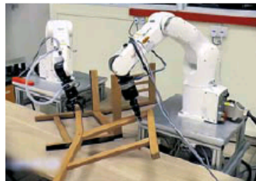
▲ Stress-free job: robots set about putting together the Stefan chair
