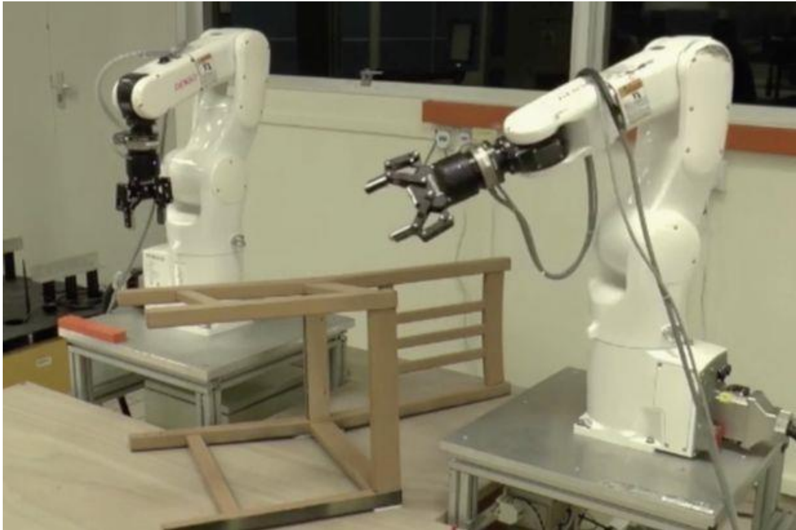
The robots were tasked with putting together an Ikea chair (Image: Nanyang Technological University)
