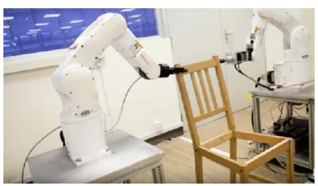
NTU'S NEW ROBOT, BUILT FROM OFF-THE-SHELF COMPONENTS, WAS ABLE TO AUTONOMOUSLY ASSEMBLE AN IKEA CHAIR IN 20 MINUTES
