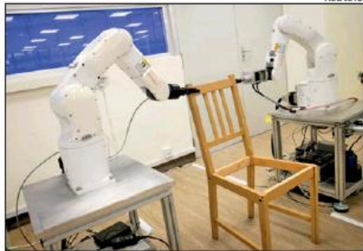
Robots assemble an Ikea chair at Nanyang Technological University (NTU) in Singapore
