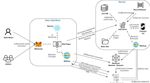
The overall architecture of the system is in the figure above, which contains user-facing web3 application, a web server that can handle HTTP requests and perform TensorFlow training, and an Ethereum with smart contract deployed.
