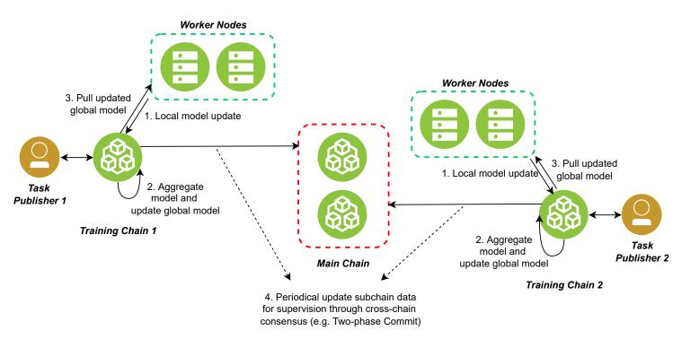
The BFEL model adopts a multi-blockchain framework. In BlockFL, the consensus nodes of the main chain are partitioned into n clusters to process FL training information from n subchains. The main feature of this design is to improve cross-chain transaction processing parallelism and throughput. It maintains security and consistency in the main chain by ensuring that every cluster can tolerate malfunctioning nodes.
