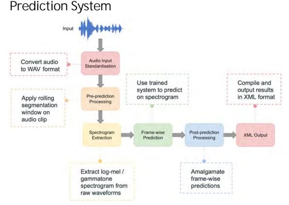
Our proposed post-prediction processing methods include frame-wise averaging and using a voting scheme. The former sums the frame-wise predictions together and then averages them based on the number of overlaps present in a particular segment. The latter sums binarized frame-wise predictions and thresholds based on the number of overlaps present.
