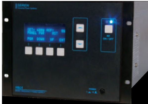
Figure 1-4: The RF Generator Control Panel
