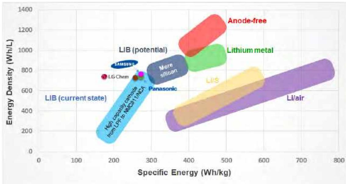
Figure 2.1.4 Energy density vs. specific energy of today's lithium-ion batteries and future battery technologies [38].
