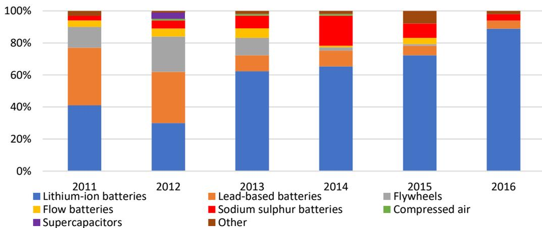
Figure 2.1.3 Technology mix of yearly installed capacity of ESS (excluding PHS) [14]
