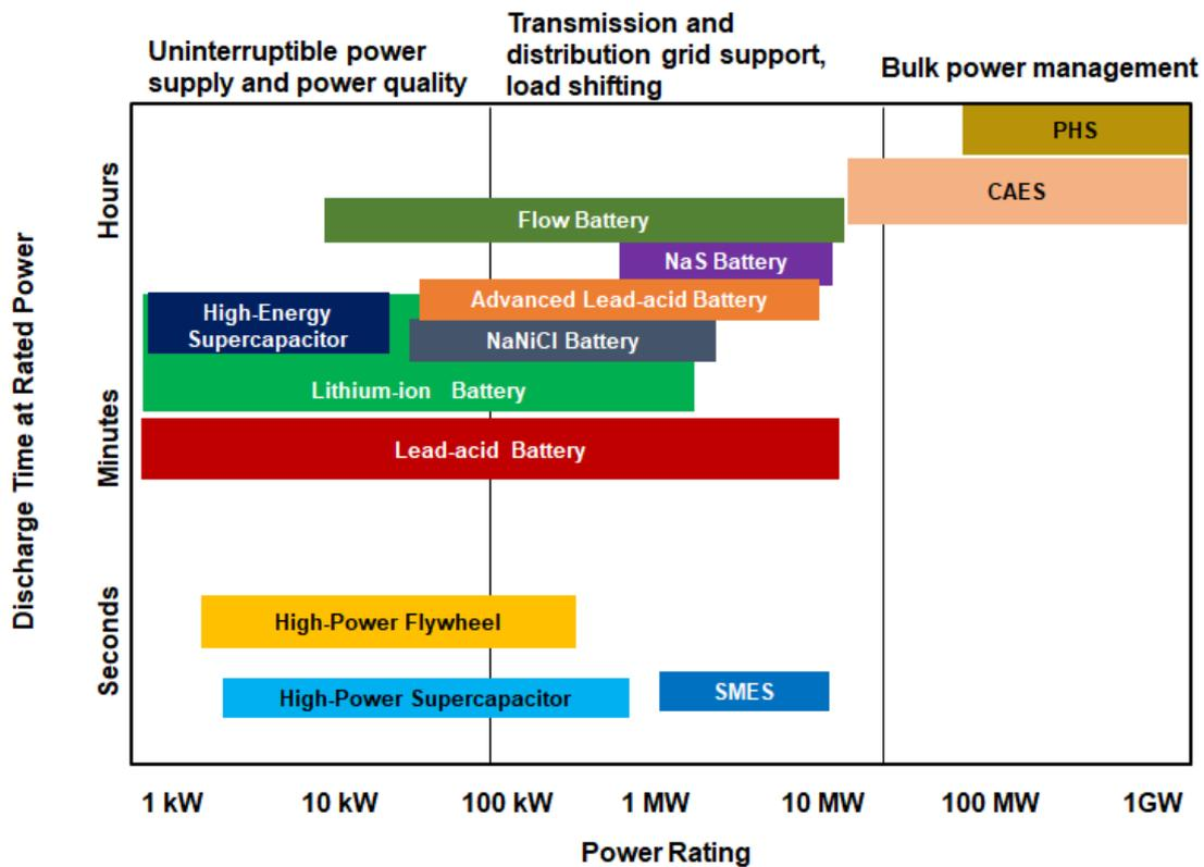
Figure 2.1.2 ESS technology suitability depending on discharge duration [13]
