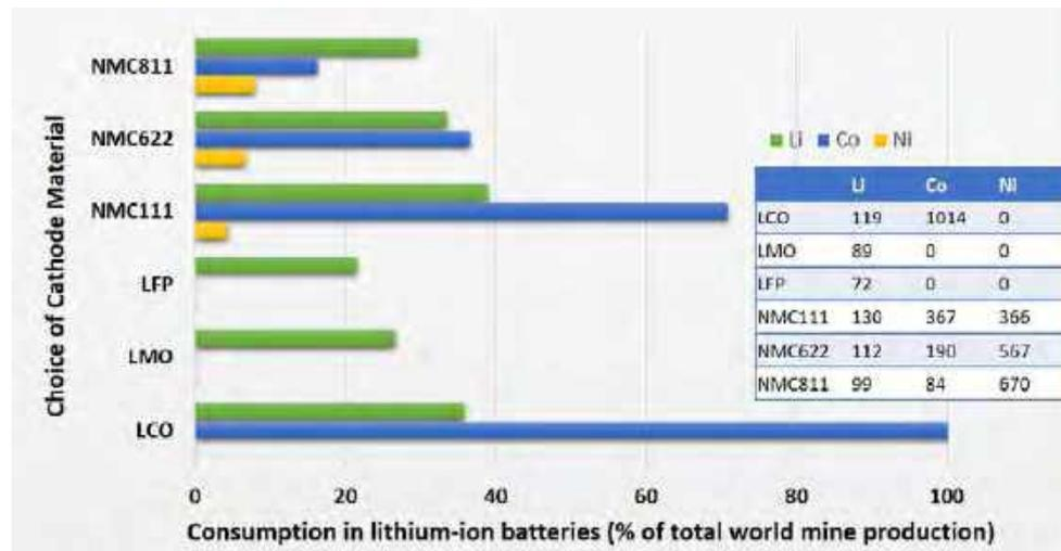
Figure 2.6.1.1 Consumption of lithium, cobalt, and nickel in the cathode of lithium-ion batteries (% of the global mine production) [76]. Note that the Co consumption for LCO exceeds 100% (~196%) and is not shown for clarity of plot. Table inset: element requirements for the corresponding cathode in units of metric ton/GWh.
