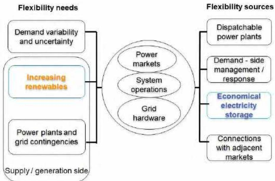
Figure 1.1 Key components of a smart flexible grid [3]
