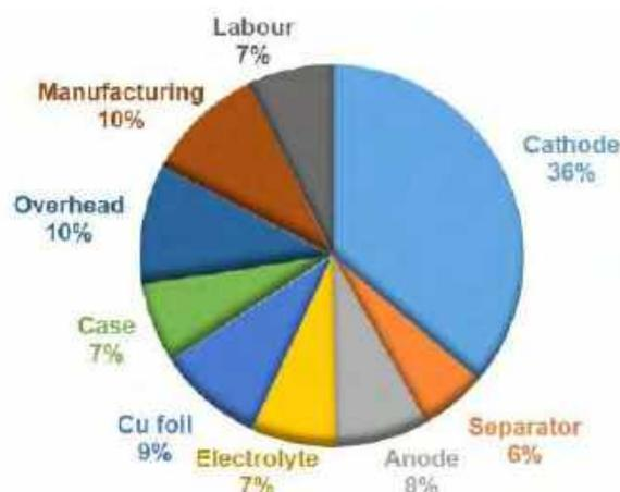
*Figure 2.6.2.1 Cost breakdown of a lithium-ion cell with NMC811 cathode [81].*
