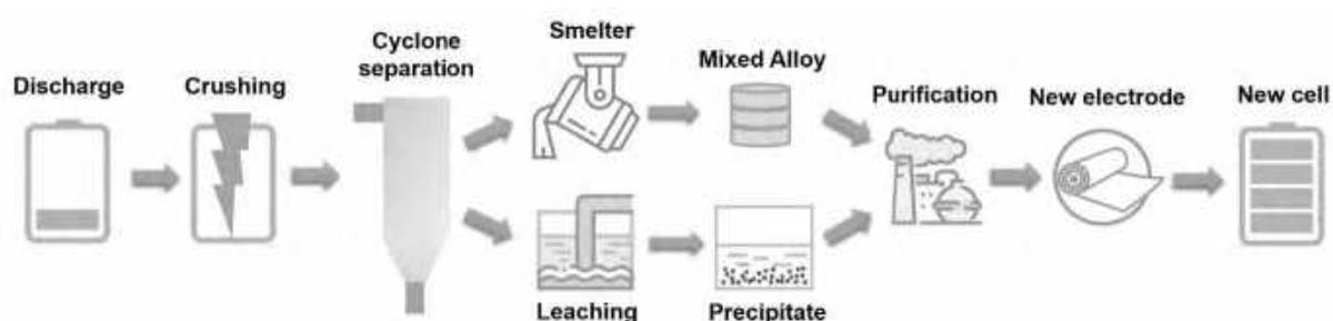
*Figure A5.2 Recycling process of lithium-ion batteries*
