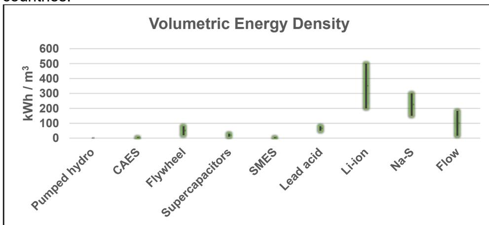
Fig. 2.4.1 Typical volumetric densities of different ESS technologies.[7], [57]–[61]
